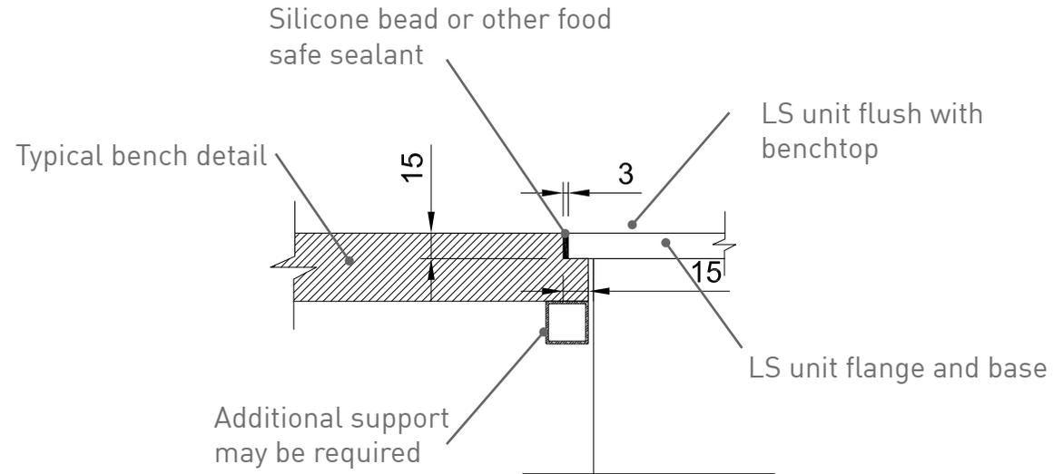
Counter top joinery must be of sufficient structural capacity to take the weight of the LS unit when the flange detail has been made.
