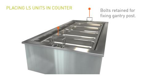
Lifting brackets are fitted to assist removing the unit from the packaging and placing into cabinetry. Use a lifting bar that can fit through the 35 x 35mm square hole. (Bar not supplied)
